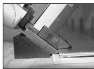
Fig. 14 Staple gun correctly positioned
