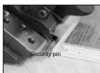
Fig. 16 Lifting the security pin over the locking element
