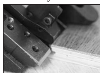
Fig. 18 Pushed in to the groove - correct position
