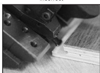
Fig. 17 Pin placed on top of the locking element
